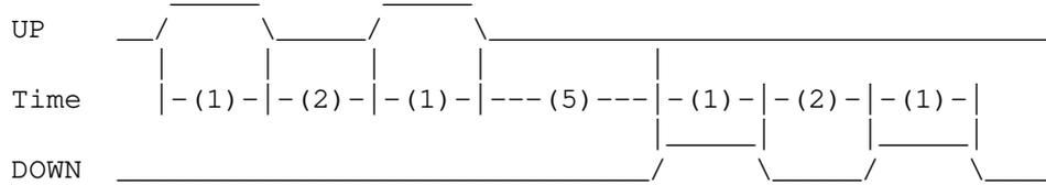
For step types 2 and higher, the exact pattern of the outputs depends on the step type (see the HAL manual for a full listing). The outputs change from one state to another at a minimum interval of **steplen**. When a direction change occurs, the minimum time between the last step in one direction and the first in the other direction is the sum of **steplen** and **dirdelay**.
