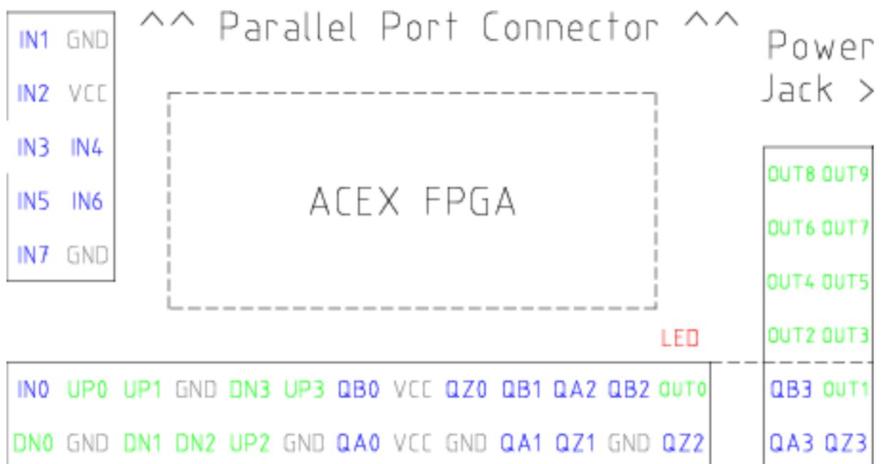
Figure 24.1: Pluto-Servo Pinout
