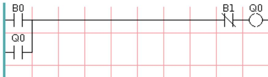
Now we have added *off* or *stop* pushbutton B1. If the user pushes it, contact from the rung to the coil is broken. When coil Q0 loses power, it drops to 0/off/false. When coil Q0 goes off, so does switch Q0, so the *holding contact* is broken, or the circuit is *unsealed*. When the user releases the *stop* pushbutton, contact is restored from the rung to coil Q0, but the rung has gone dead, so the coil doesn't come back on.
