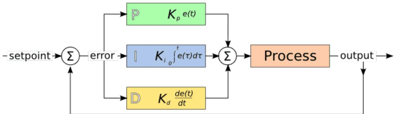
Figure 1.2: PID Loop
