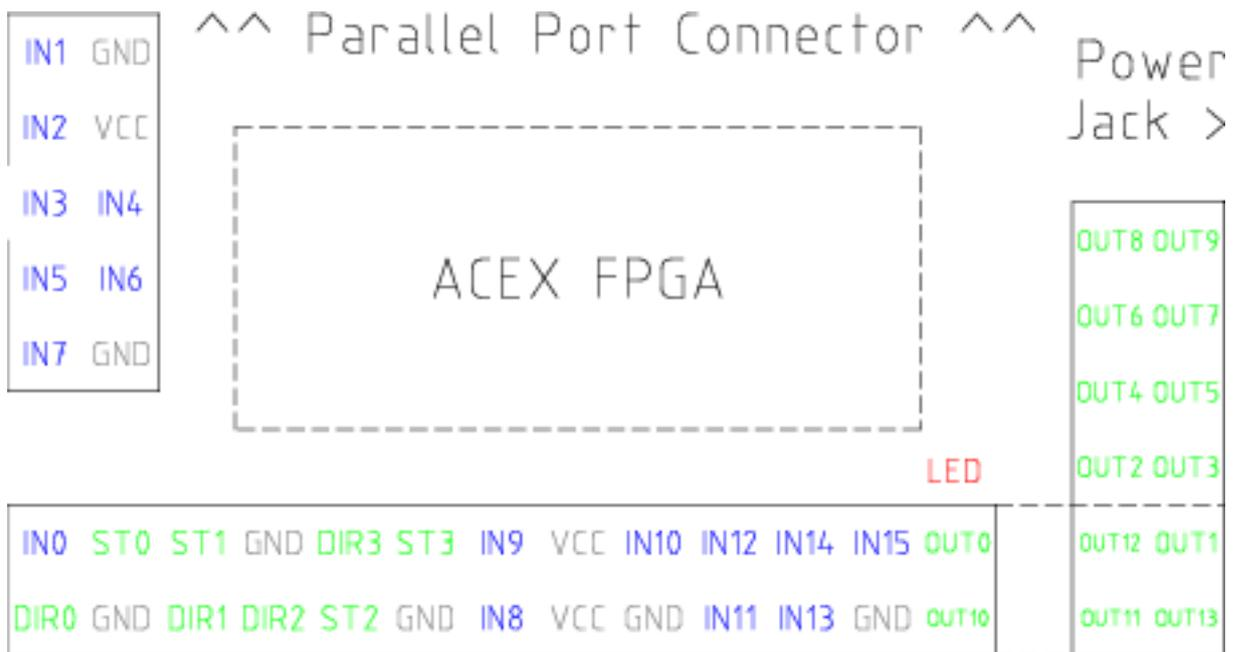
Figure 24.2: Pluto-Step Pinout
