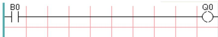
The input on the left, B0, a normally open contact, is connected to the coil (output) on the right, Q0. Now imagine a voltage gets applied to the leftmost end, because the input B0 turns true (e.g. the input is activated, or the user pushed the NO contact). The voltage has a direct path to reach the coil (output) on the right, Q0. As a consequence, the Q0 coil (output) will turn from 0/off/false to 1/on/true. If the user releases B0, the Q0 output quickly returns to 0/off/false.
