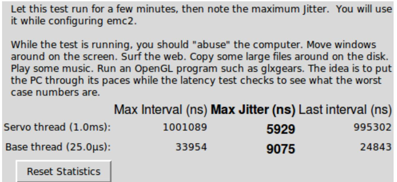
Figure 2.1: HAL Latency Test
