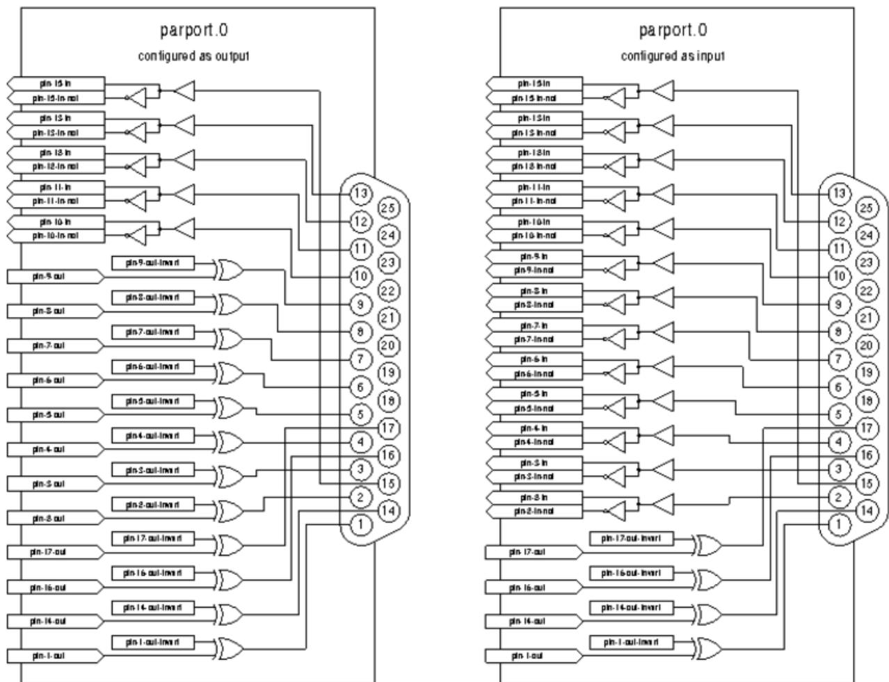
Figure 17.1: Parport Block Diagram
