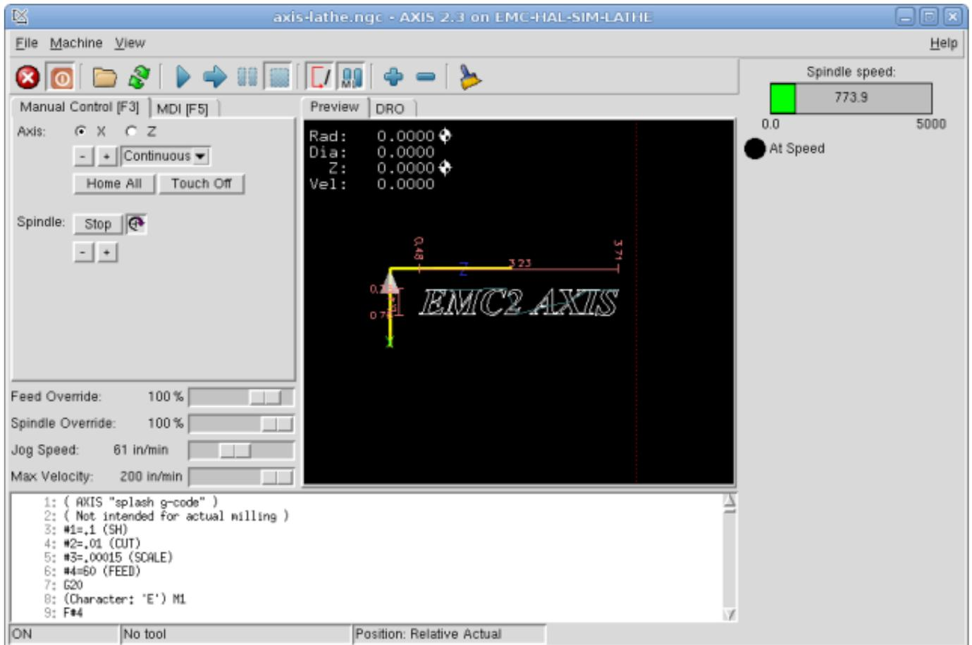
This is what the newly created PyVCP panel should look like in AXIS. The *sim/lathe* configuration is already configured this way.
