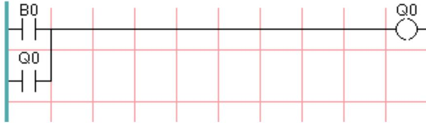
As before, when the user presses pushbutton B0, coil Q0 comes on. And when coil Q0 comes on, switch Q0 comes on. Now the interesting part happens. When the user releases pushbutton B0, coil Q0 does not stop as it did before. This is because switch Q0 of this circuit is effectively holding the user's pushbutton pressed. So we see that switch Q0 is still holding coil Q0 on after the *start* pushbutton has been released.
