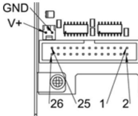
Figure 27.6: Pin numbering of homing & end switch connector
