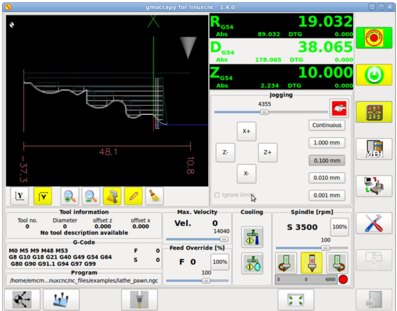
Figure 2.14: Back Tool Lathe
